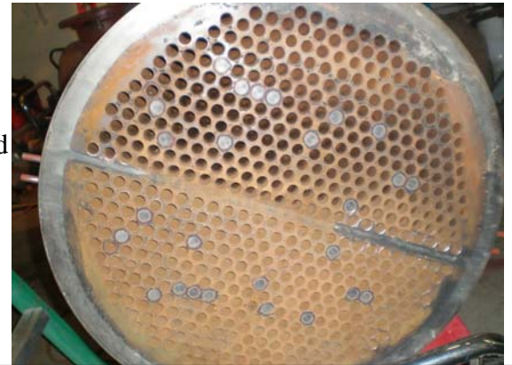
Each of the silver dots indicated a failed tube
